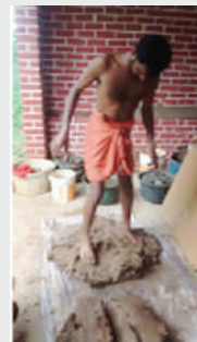
Leg pugging to make the clay uniform
