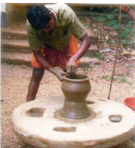
Shaping of pot using manual potter's wheel
