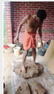
Leg pugging to make the clay uniform
