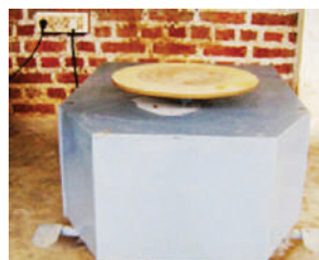
Motorised potter's wheel developed at IRTC
