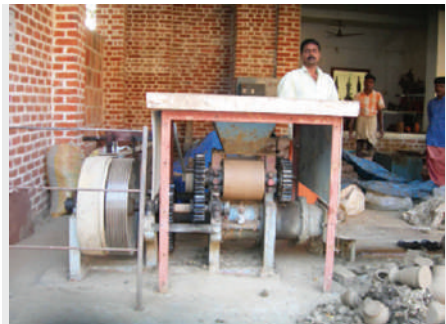
Pugmill installed at IRTC capacity : 1 ton/day, Power – 10 HP
