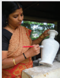
Giving a coating of cement primer on the pot
