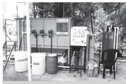
Moving Bed Biofilm Reactor Technology (MBBR)
